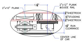
NOTE: WHEN STUD AND SHEETROCK CONSTRUCTION IS USED ON THE GUIDE RAIL SUPPORT WALL 4"x4" STUDDING IS NEEDED BEHIND THE 2"x12" PLANK.
