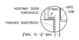
DOOR SILLS TO BE INSTALLED BY GC AFTER THE LIFT SUPPLIER HAS INSTALLED A RUNNING PLATFORM. SILL MUST BE BROUGHT OUT TO NOT LESS THAN ½" AND NOT MORE THAN 1 ¼" TO THE RUNNING PLATFORM WHILE MAINTAINING A DISTANCE OF 3" FROM THE HOISTWAY FACE OF THE LANDING DOOR (OR GATE) TO THE HOISTWAY EDGE OF THE LANDING SILL.
