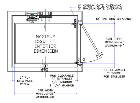
The following specs are to be provided by the General Contractor (GC), except as noted, prior to Elevator Contractor (EC) installing the elevator equipment.
